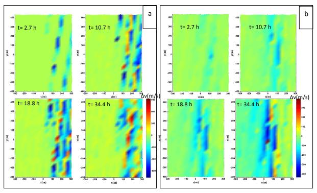
*Figure:* time-lapse velocities along x-direction (a) and the y-direction (b) during hydraulic fracturing in the modeled reservoir. The plotting area is about 410m by 830m corresponding to the area of receiver particles.
