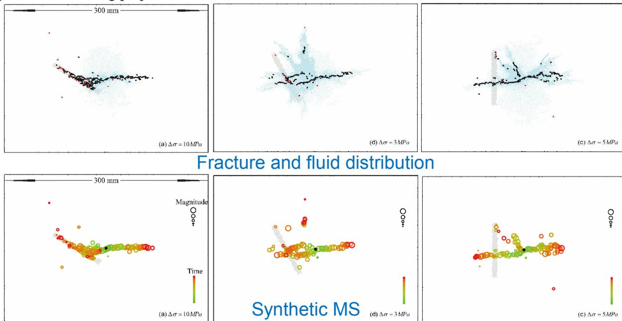
**Figure:** Interaction as shown in Arrestment, Dilation and Crossing between natural and hydraulic fractures with the variations of in-situ stress and interaction angles.
